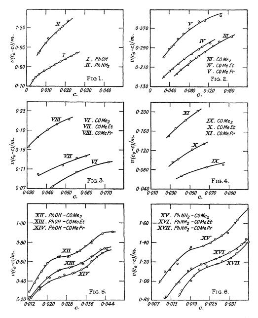
The adsorption of phenol from phenol-ketone solutions containing the ketone initially at concentration 0.217 g.-mol./l. is represented in Fig. 5, and of aniline from aniline-ketone solutions of initial ketone concentration 0.206 in Fig. 6.
